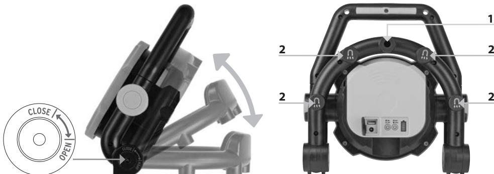
For set-up, the battery-operated lamp can be unfolded to several settings, but, at most, to the "OPEN" marking. Do not force the lamp further open since this would damage the mechanism! The lamp can be hung up on a hook on the frame using the mounting opening (1) or on a metal surface using the magnets (2). Please make sure the surface is stable in order to avoid damage to the product or injuries to persons!
